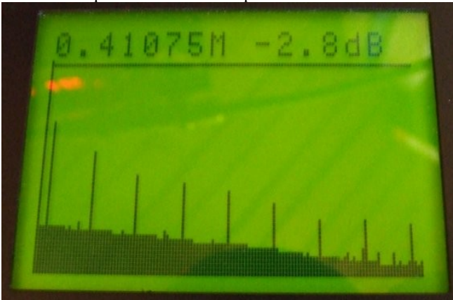
Monitor – square wave 1 MHz spectrum
