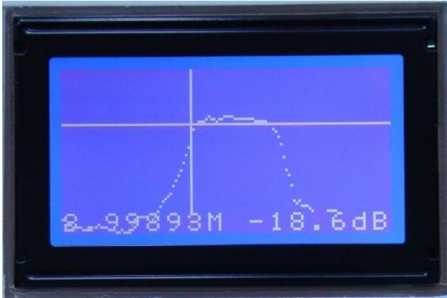
In band measure – narrowband x-tal filter
