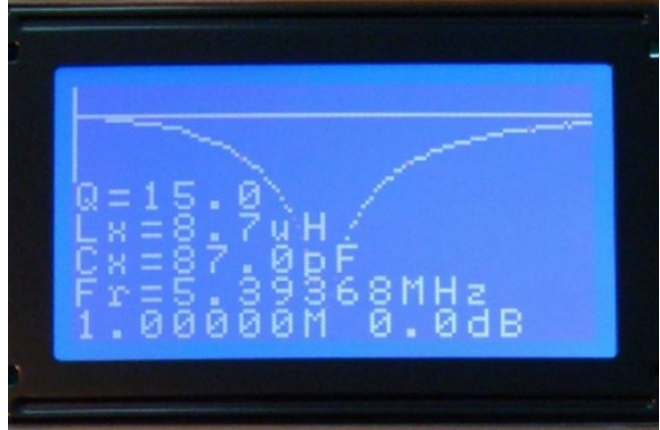
LCQ – measure of serial resonance circuit about 5.3 MHz
